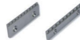
**Grip ledge** fits step jaw order no. 01.25.150.008, order no. 01.25.150.009 for improved hold of the workpieces on the step (4.5 mm deep, 2.5 mm wide)
