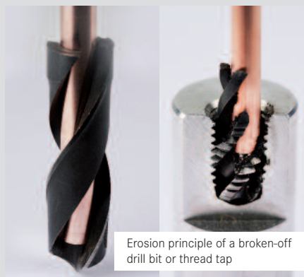
Erosion residue of a broken-off drill bit after erosion process with electrode in special length 500 mm
