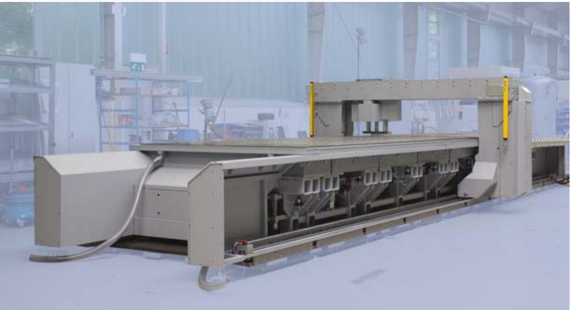
Vacuum clamping fixture incl. gantry and hydraulic press (2 tons) for selective pressing of large aluminium work pieces.
