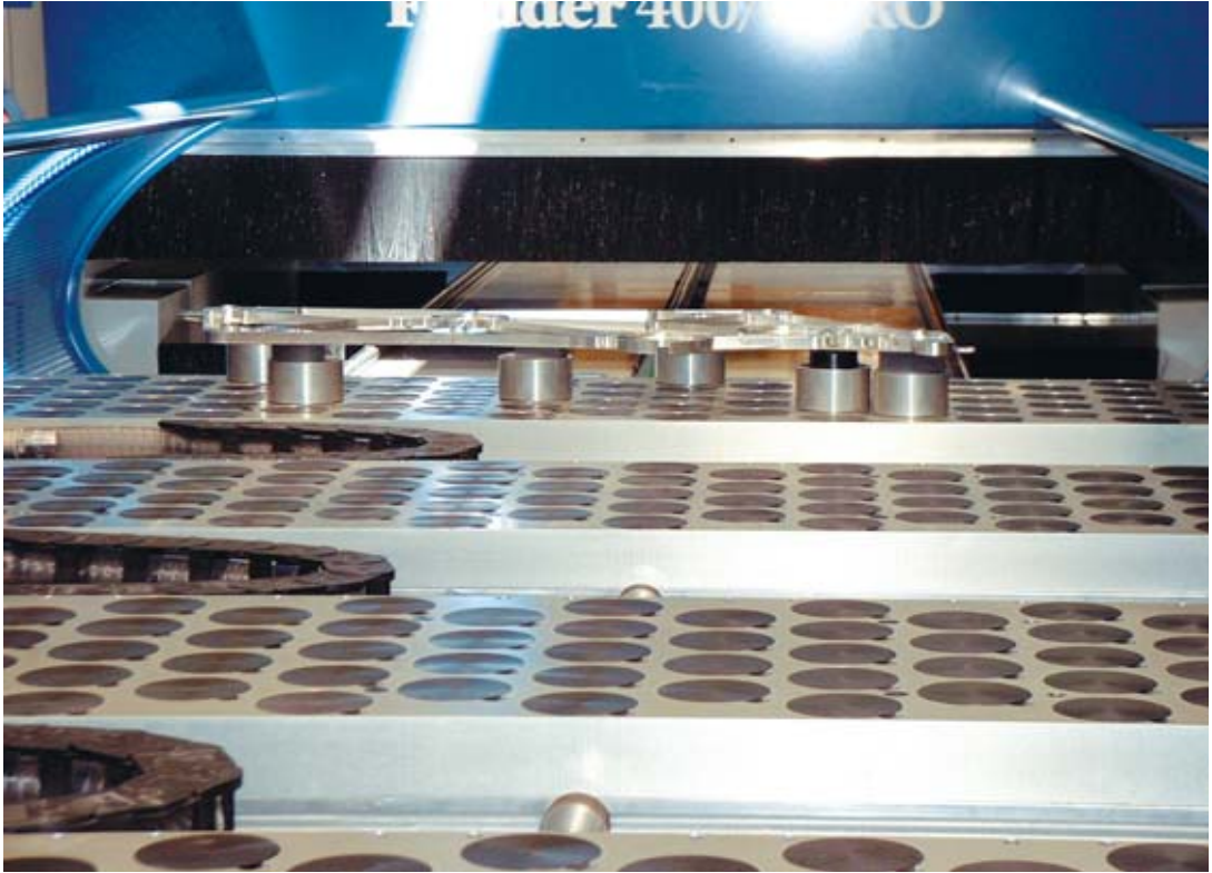
FLIP-POD™-clamping system for a CNC deburring machine, used on aeroplane parts
