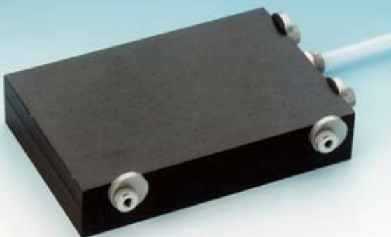
Perforated-grid chuck with eccentric end stops
