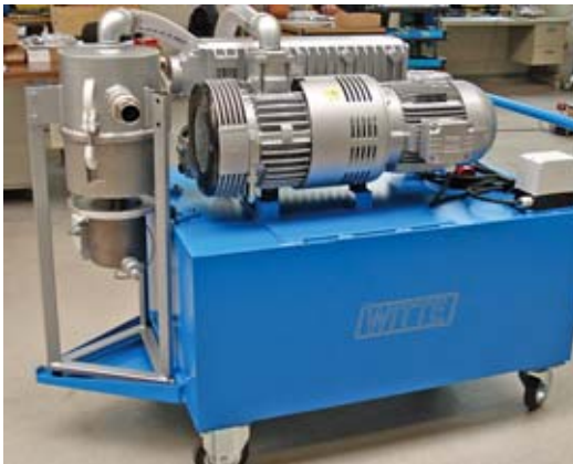
Vacuum unit with automatic liquid separator, see also p. 87
