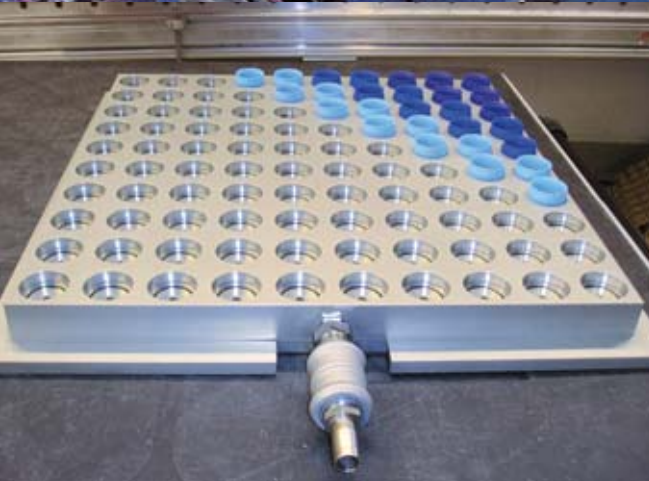
Vacuum clamping chuck for bottle caps as used in quality control.
