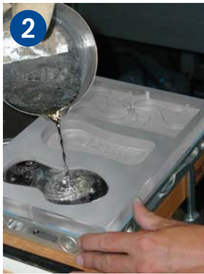
Right: Filling hollow with melted Witte Weiguss alloy
