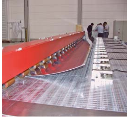
Clamping fixture for machining cylindrical pre-formed aircraft fuselage parts (13m x 4,10m) Parts are pressed down, rolled flat and clamped using vacuum as well as pneumatic and hydraulic clamps
