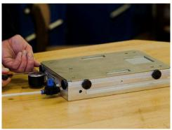
The workpiece is fixed using the adjustable eccentric stops.
