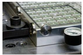
The height-adjustable eccentric stops absorb the sliding forces, and can be adjusted individually to the workpiece height.
