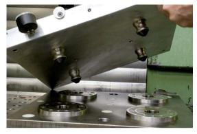
Alternatively, the vacuum clamping plate can be integrated into the AMF "Zero-Point" clamping system (see the AMF catalogue "Zero-Point Systems") without difficulty through the existing receiving holes ( K20 ).
