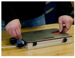
The workpiece to be processed is placed on it and fixed using the adjustable eccentric stops.
