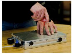
The adapter plate is screwed to the vacuums clamping plate
