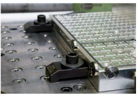
The vacuum clamping plate can be fastened through lateral grooves or the mounting holes.
