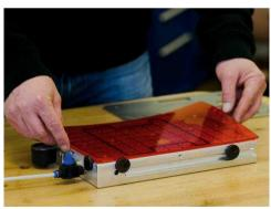
The adapter mat is placed onto the vacuum clamping plate.
