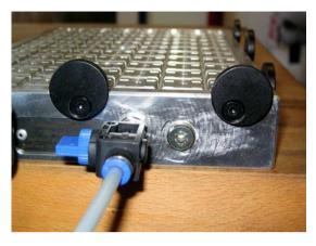
Plug the pneumatic hose  $\emptyset$  6 mm into the shut-off valve 1.
