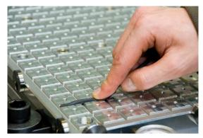
The sealing cord is placed into the grid of the vacuum clamping plate.
