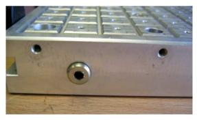
Seal this opening with a blanking screw 2.
