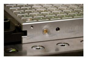
Orient the vacuum clamping plate on the machine table
