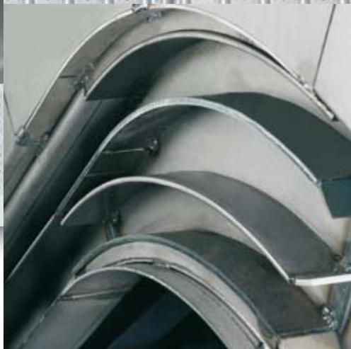
Each frame is designed to withstand the forces it will see in tough machining applications. Hardened track is used in all high wear areas, such as the curves, to provide long conveyor life. All curves and tails are smoothly transitioned so chips have no areas to accumulate in.
