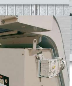
The upper conveyor separates heavy chip loads from the coolant stream. This conveyor efficiently removes chunks, stringy, bushy and large chips and is ideal for multiple material applications. Any small chip or particle passing through the upper conveyor is trapped in the lower filtering conveyor. High speed aluminum machining is one of the many applications ideal for the Turbo MF2/MF3.
