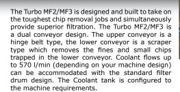
LNS's Turbo MF2/MF3 was designed with the increase in coolant flow in mind. Large diameter filter drums provide coolant flow of up to 570 I/min matching the needs of high flow pumps to any machining requirement.
