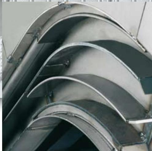
Turbo HB conveyors come in a variety of frame types that are matched to the size limitations and horse power of the machine tool. Belt designs are flexible to match specific chip geometry and coolant requirements.
