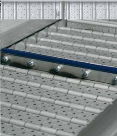
Each belt has a minimum of 2 wiper cleats that clean chips that have washed into the inside of the conveyor frame. Because all conveyor transitions use a smooth radius, these wipers do an excellent job of keeping the frame free of chips, reducing the risk of a belt jam. All belt rollers and pins are hardened for durability. For extreme wear conditions on super heavy duty conveyors, hardened rollers mounted on hardened bushings are used with double link plates for maximum belt strength.
